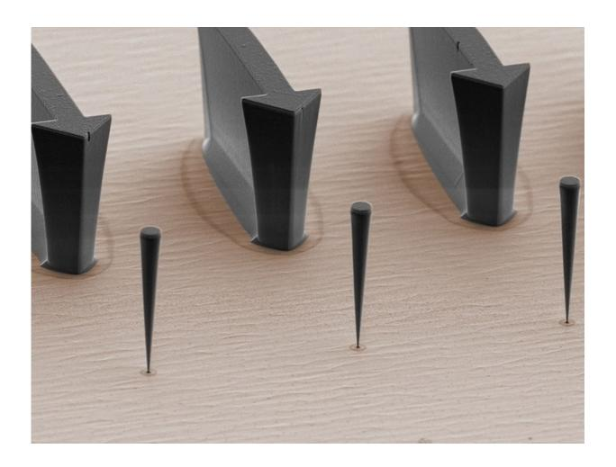
Trumpet-shaped nanowires with a length of about 10 micrometers are coupled to quantum dots located at their bases. The movement of the nanowire can be detected with a sensitivity of 100 femtometers by changing the wavelength of the light emitted by the quantum dots. The arrows are important for fabrication and help to locate the nanowires. Credit: Grenoble Alps University
