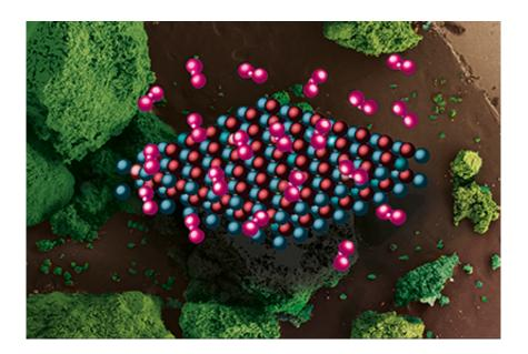
This electron microscopy image of concrete includes a model of sulfur dioxide interactions with concrete surface – represented by the colored spheres. Credit: Marija Illoska
