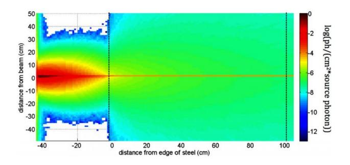
This image shows how a compact, precise photon beam (red line) could penetrate through 40 centimeters of steel (left side of image). The beam could be useful for detecting and identifying nuclear materials, among other uses. Credit: Berkeley Lab, University of Michigan
