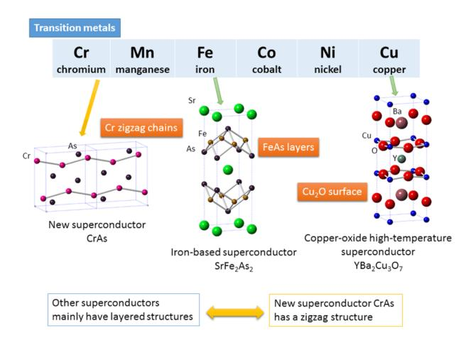
Figure 1: Crystal structures of the new superconductor, an iron-based superconductor, and a high-temperature copper-oxide superconductor
