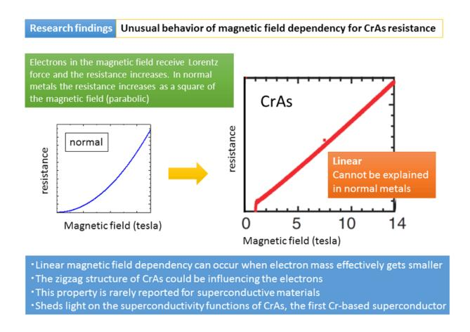
Figure 2: Graph of the magnetic field dependence of electronic resistance for CrAs
