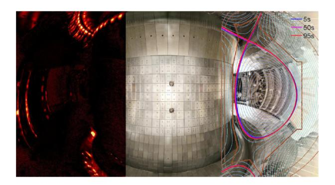
Basic parameters of the world's longest 101.2 s high confinement discharge achieved on EAST (Bt=2.5T, PRF=3.0MW, ne/neGW=0.55, Te=4.0KeV, H98y2=1.1, Upper single null configuration) Credit: EAST Team
