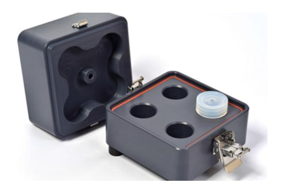
The Mixed Odor Delivery Device contains four compartments in the base (right), each with an odor regulating lid, that releases odors to mix into the top (left) to be expelled and tested with canine units. Photo Credit: NRL Tech Transfer Office
