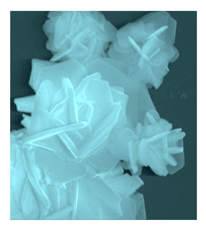
A scanning electron microscope image shows a flake of the two-dimensional electrocatalyst developed at Rice University. The material made of a transition metal and sulfur proved able to extract hydrogen from water with high performance and low cost. Credit: Yakobson Group/Rice University
