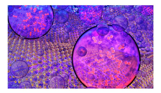
Hydrogen gas bubbles evolve from water at tantalum disulfide electrocatalyst surfaces. Catalytic activity in layered metal dichalcogenides like these is usually limited to edges, but this work reports new materials that also can generate hydrogen at the surfaces. Credit: Ryan Chen/LLNL.
