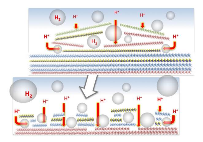
An electrocatalyst created at Rice University proved as effective as platinum for the production of hydrogen. The process creates hydrogen bubbles between planes of the layered material, which breaks the layers up and makes catalytic sites more accessible. Credit: Yuanyue Liu/Rice University
