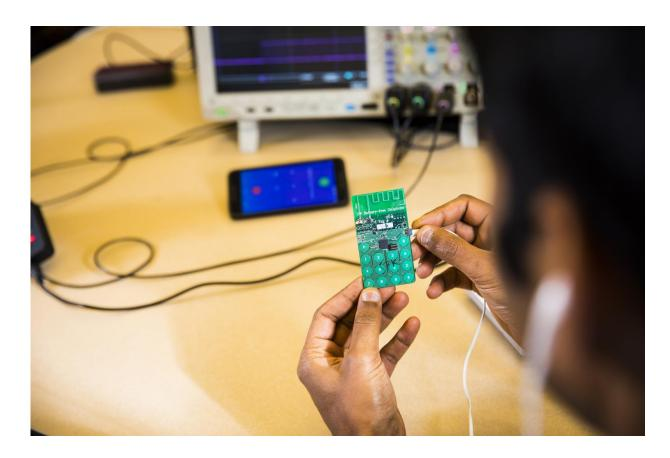
The battery-free phone developed at the UW can sense speech, actuate the earphones, and switch between uplink and downlink communications, all in real time. It is powered by either ambient radio signals or light. Credit: Mark Stone/University of Washington
