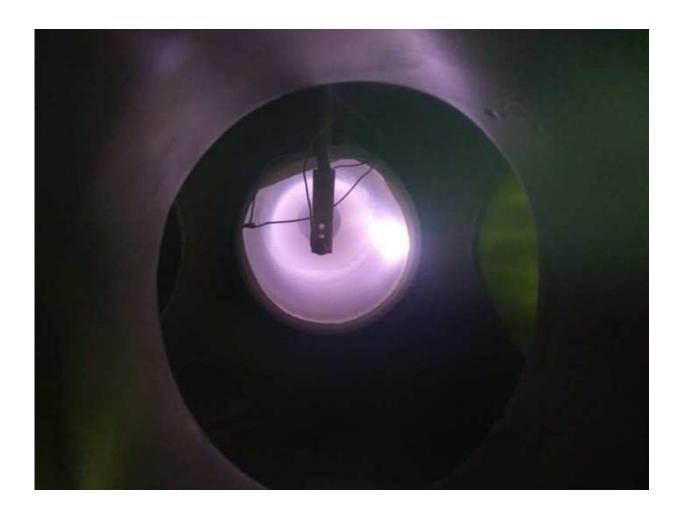
A localized glow region, the complex space charge configuration, near cathode surface with application of ~28G magnetic field. Credit: Shaw et al/AIP Publishing
