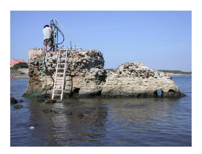
ROMACONS drilling at a marine structure in Portus Cosanus, Tuscany, 2003. Drilling is by permission of the Soprintendenza Archeologia per la Toscana. Credit: J.P. Oleson
