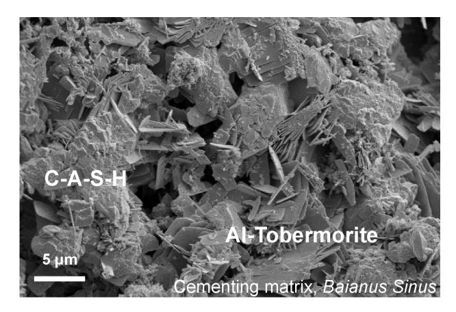
This microscopic image shows the lumpy calcium-aluminum-silicate-hydrate (C-A-S-H) binder material that forms when volcanic ash, lime, and seawater mix. Platy crystals of Al-tobermorite have grown amongst the C-A-S-H cementing matrix. Credit: Marie Jackson.
