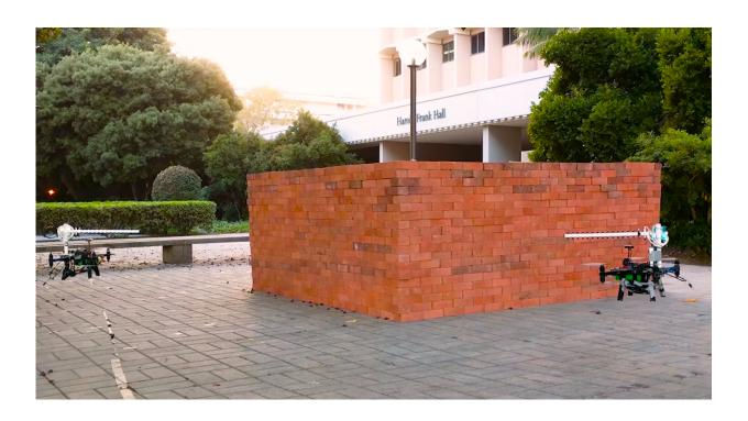
Researchers at UC Santa Barbara professor Yasamin Mostofi's lab have given the first demonstration of three-dimensional imaging of objects through walls using ordinary wireless signal. The technique, which involves two drones working in tandem, could have a variety of
