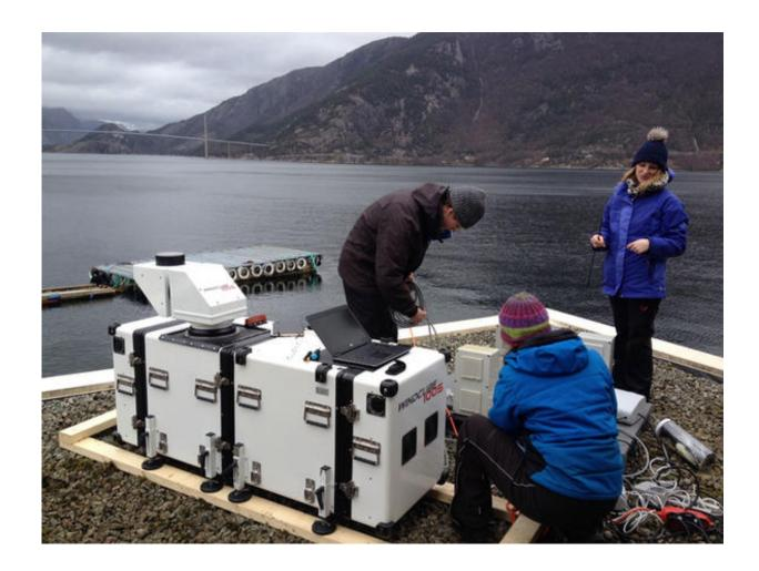
Researchers in the field preparing a long-range lidar laser instrument called WindCube100S, deployed at the Lysefjord center. The Lysefjord bridge is in the background. Jasna B. Jakobsen (seen from behind) and Etienne Cheynet, both from UiS, and Valerie Kummer from UiB. Credit: Benny Svardal / CMR
