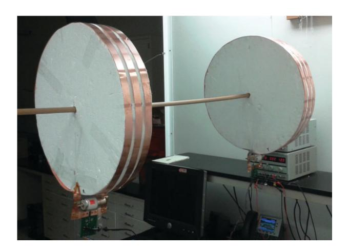
Stanford scientists have created a device that wirelessly transmits electricity to a movable disc. The technology could some day be used to charge moving electric vehicles and personal devices. Credit: Sid Assawaworrarit/Stanford University
