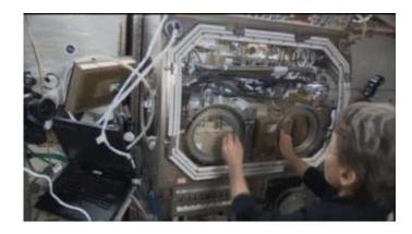
The new fully-removable front window of the Microgravity Sciences Glovebox allows for quicker payload removal and set-up. Credit: NASA
