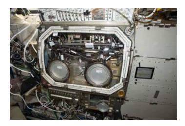
The Microgravity Science Glovebox on the International Space Station with the new window installed. The new latch system can be seen around the outside of the window, allowing for easy removal and access to the inside of the glovebox. In this image, the glovebox is filled to capacity with the Packed Bed Reactor Experiment. Credit: NASA
