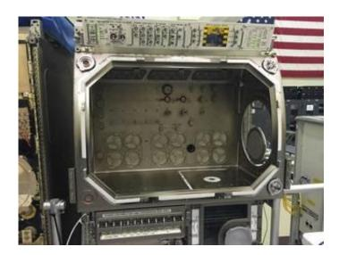
The engineering model of the Microgravity Science Glovebox at NASA's Marshall Space Flight Center, which manages the facility, with the front window removed, showing the space and access available inside. Credit: NASA
