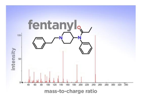
The mass spectrum for the synthetic opioid, fentanyl. The mass spectrum is like a molecular fingerprint, and is used to identify unknown compounds. The red lines represent the charged fragments of the molecule created during analysis. The vertical axis shows the relative intensity, or amount, of each fragment, while the horizontal axis shows the mass-to-charge ratio for each fragment. Credit: NIST
