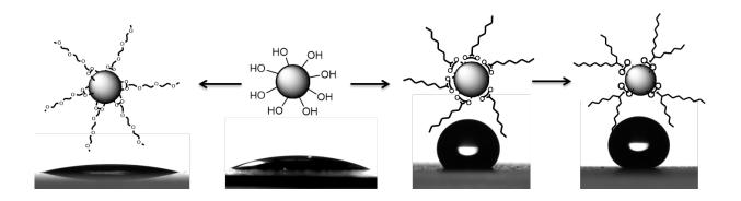
A schematic of the functionalization of the nanoparticles along with photographic images of the water droplets on spray-coated microscope slides. An environmentally friendly superhydrophobic coating to superhydrophilic coating for antifogging and antifouling according to scientists at Swansea University. Credit: Shirin Alexander Swansea University
