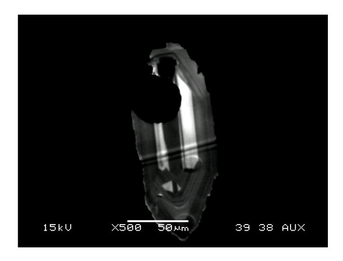
A zircon crystal from an eruption at Mt. Tarawera, New Zealand, about 700 years ago. The hole at upper right is where a piece was removed with a laser. The chemical profile across the crystal reveals the conditions under which it formed and survived in the magma chamber. Credit: Allison Rubin
