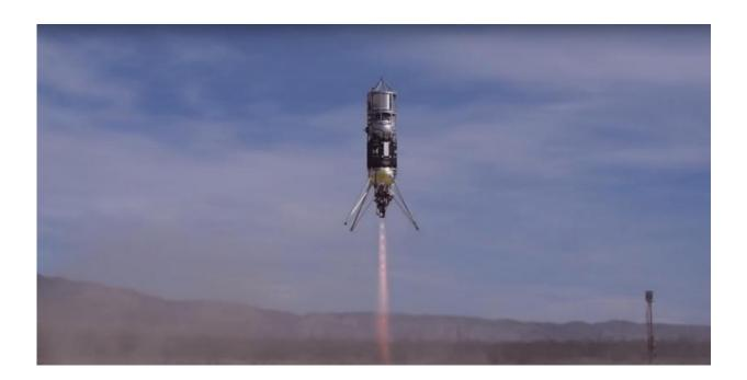
A rocket flying several landing technologies was recently flown in the Mojave Desert. These flight tests, coordinated by NASA, are helping to develop technology for precise landings in uneven terrain. Image Credit: NASA/JPL-Caltech
