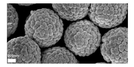
Scanning electron microscope (SEM) image of the silica raspberry-like particles, showing the controlled roughness of their surfaces. Credit: Michele Zanini, Isa Group, ETH Zurich
