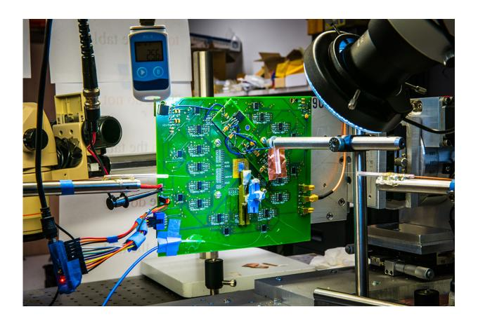
At Caltech, engineers have developed a new camera design that replaces the lenses with an ultra-thin optical phased array (OPA). Credit: Caltech
