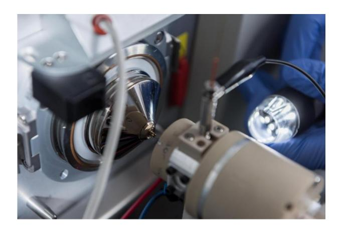
The DRILL device is connected to a mass spectrometer to sort charged droplets and improve desolvation of ionized biomolecules for analysis. The device requires no modification of the mass spectrometer, and can be accommodated within the standard work flow now used by researchers. Credit: Rob Felt, Georgia Tech
