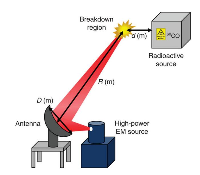
Schematic of a possible setup for the detection of radioactive material inside a container. Credit: UNIST
