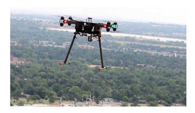
NIST has combined a laser instrument that 'combs' the air with a flying multicopter to scan and map atmospheric gases over kilometer distances. Credit: NIST
