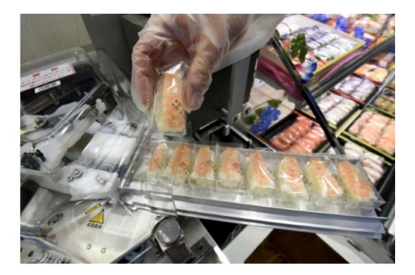
Suzumo Machinery is showing off a device that combines rice, spicy green wasabi paste and fresh fish before wrapping the sushi in a clear plastic wrap stamped with an expiration date - at a rate as quick as 2,000 pieces an hour
