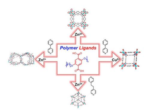
y combining different metal atoms (for example zinc, Zn, or copper, Cu) with the molecular polymer chains (or ligands), scientists can control the resulting structure. By controlling the structure, scientists can design a structure that can separate mixed gases (for example, trapping carbon dioxide and not nitrogen). Credit: Prof. Seth Cohen, University of California, San Diego
