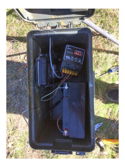
Electricity gathered by the solar panel is stored by a 12V deep cycle battery. A Raspberry Pi minicomputer records tag ping data. Credit: Vince Voegeli
