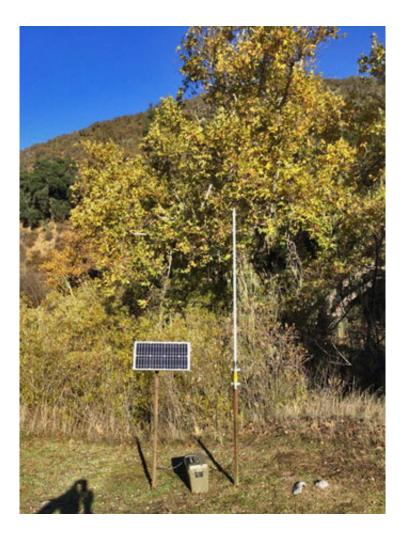
Tag pings are detected by base station antennas. The most recent design of the base station runs on solar power and can be moved easily to a sunny spot near a woodpecker granary. Credit: Vince Voegeli
