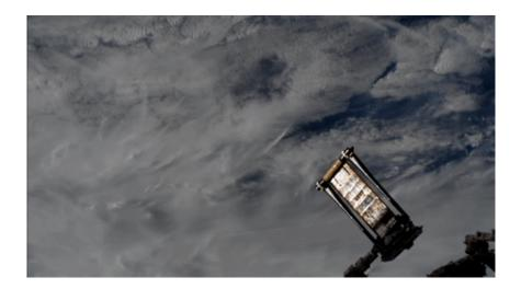
The Roll-Out Solar Array (ROSA) was deployed from the end of the Canadarm2 robotic arm Sunday, June 18 outside the International Space Station. ROSA is an experiment to test a new type of solar array that rolls open in space like a party favor and is more compact than current rigid panel designs. Credit: NASA
