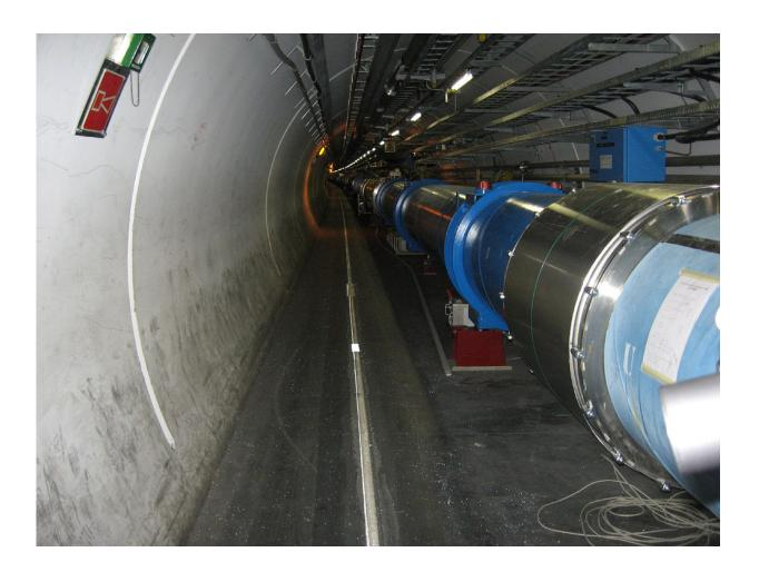
Large Hadron Collider dipole magnets. Credit: CERN
