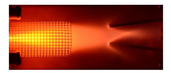
As the skimmer temperature is lowered, the density of the beam rises. Pulsed discharged enabled the researchers to visualize the beam density. Credit: Weizmann Institute of Science
