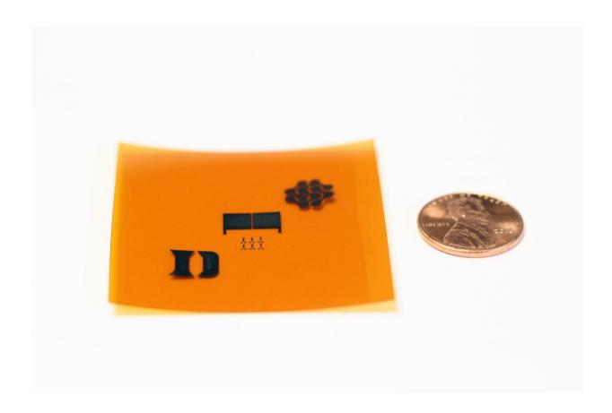
Demonstration of the printed carbon nanotubes on a flexible surface. The prototype tire tread sensor (middle) is flanked by the logos of Duke University and Fetch Automotive Design Group. Credit: Amanda Dixon, Duke University
