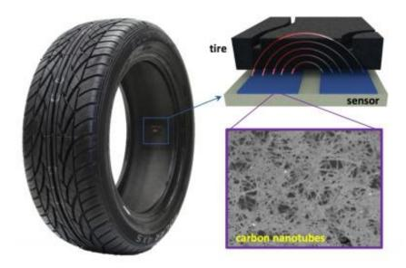
Illustration of how the novel tread sensor works. The sensor is placed on the inside of the tire, where the tire wall and tread interferes with an electric field that arcs between two electrodes. That interference can be measured to determine the thickness of the rubber with millimeter accuracy. Credit: Joseph Andrews, Duke University
