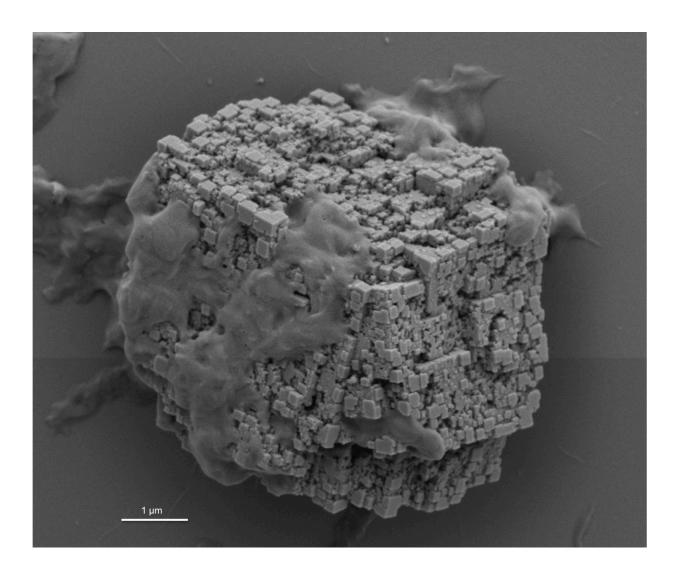
Scanning electron microscopy image of a calcite crystal generated in the presence of the sea urchin protein rSpSM50 on a silicon wafer showing organized nanotexturing on exposed surfaces. Credit: NYU Dentistry: Evans
