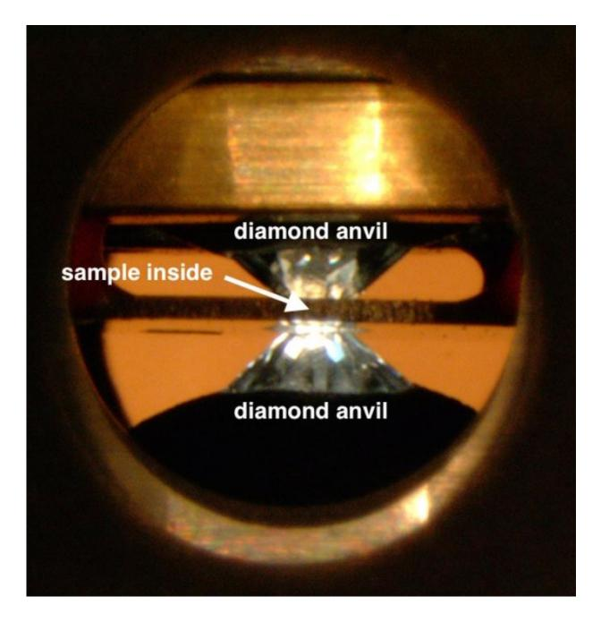
To subject the bridgmanite sample to high pressures, it is held between two anvils made of gem-quality diamond. Credit: Dan Shim
