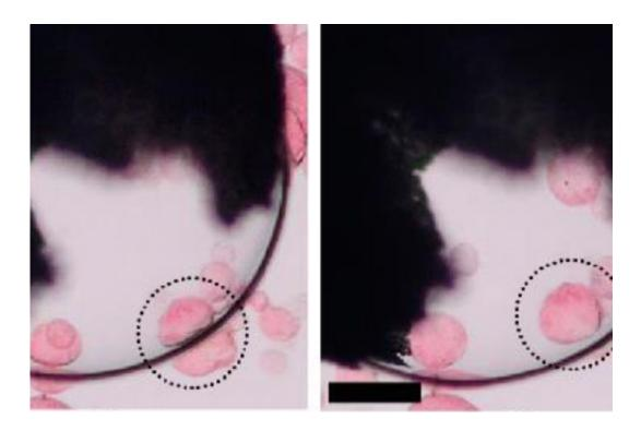
Time sequence of optical microscopy images showing spontaneous transfer of a dye-loaded cross-linked silica colloidosome (red object, dotted line) into a magnetic emulsion droplet through a fatty acid stabilized aperture. Scale bar =  $100 \mu m$ . Credit: University of Bristol
