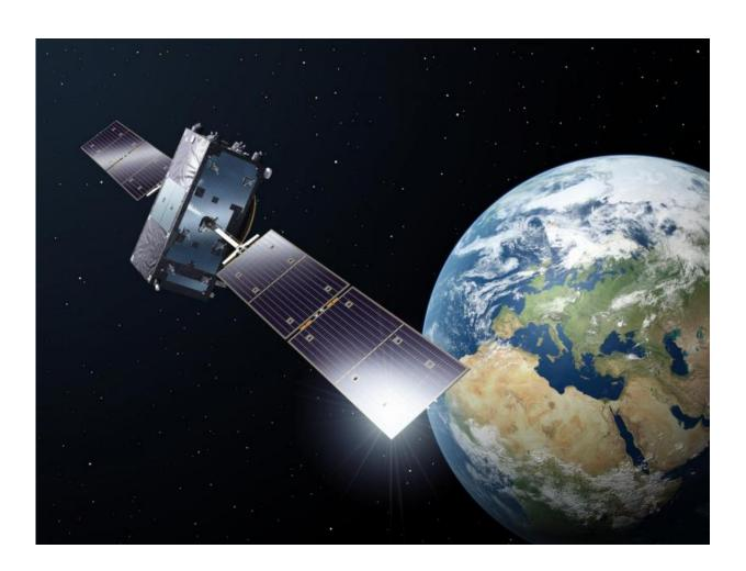
Galileo satellites are placed in medium orbits, at 23 222 km altitude along three orbital planes so that a minimum of four satellites will be visible to user receivers at any point on Earth once the constellation is complete. The fifth and sixth Galileo satellites, launched together on 22 August 2014, ended up in an elongated orbit travelling out to 25 900 km above Earth and back down to 13 713 km. In addition, the orbits are angled relative to the equator less than
