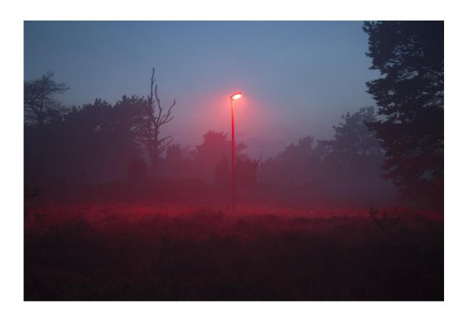
The red light posts are placed in otherwise undisturbed natural areas, to be able to measure the effect of light pollution. And to compare the differences between different colours of light. Credit: Kamiel Spoelstra / NIOO-KNAW
