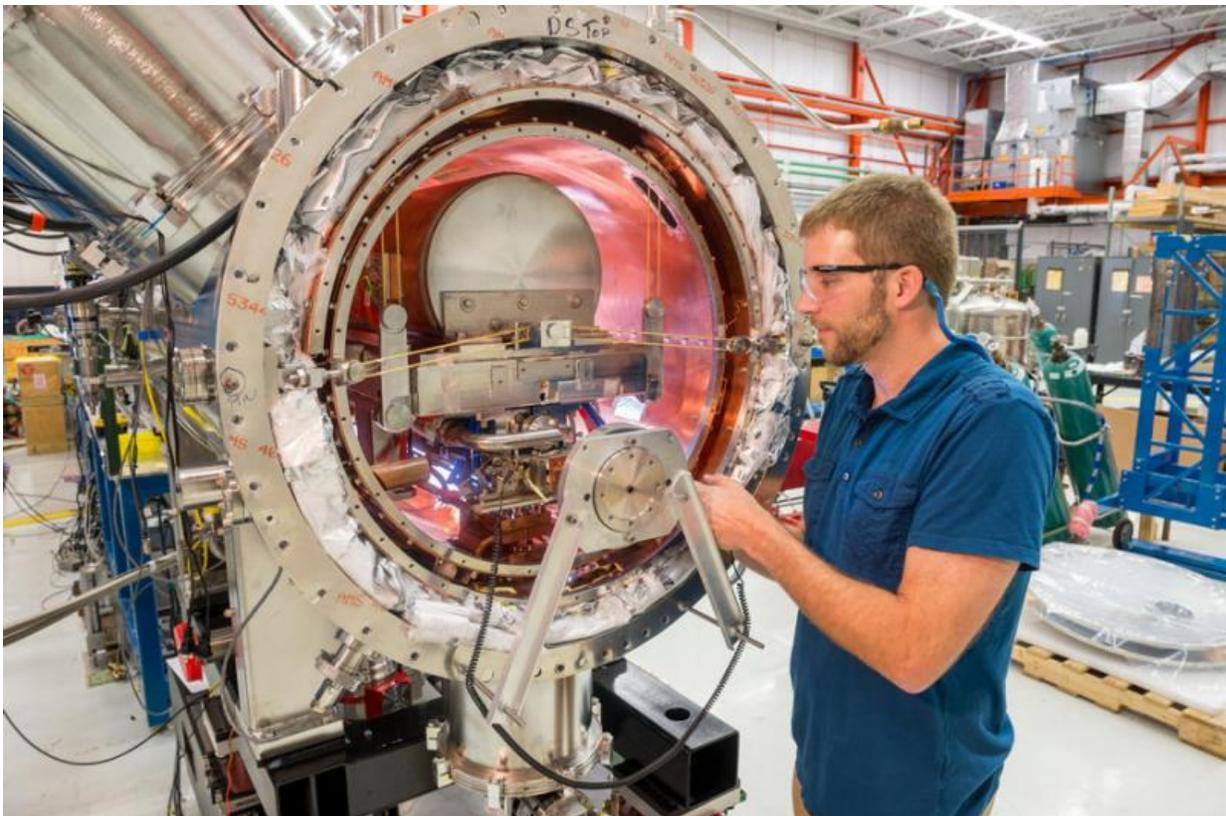
Argonne and Berkeley national laboratories have collaborated to design, build and test two superconducting undulator devices that could make X-ray lasers more powerful, versatile, compact and durable. Above: Argonne Accelerator Systems Division engineer Matt Kasa checks the instrumentation of the undulator. Credit: Argonne National Laboratory
