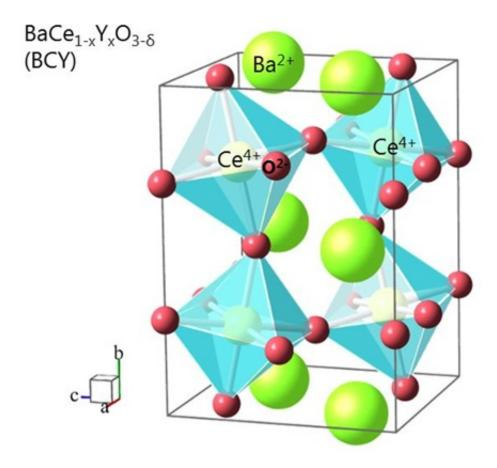
The experiments have been conducted with Barium ceric oxide. The crystal is non conductive in a dry state. When moisture comes in, the protons form OH-bondings and move through the crystal. Credit: Swiss Federal Laboratories for Materials Science and Technology
