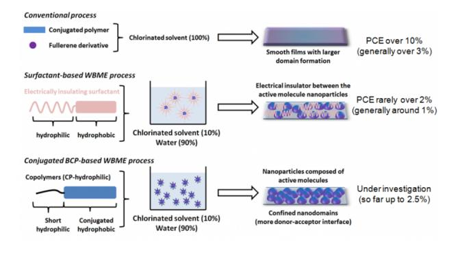
Fig. 2: Schematic comparison of thin film morphology and device performances of active layers prepared using conventional spin-coating from chlorinated solvents, recently introduced water-based micro-emulsion processes and water-based micro-emulsion process developed at UEC. Credit: University of Electro Communications
