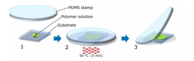
Fig. 1 Push coating devices onto substrates with polydimethylsiloxane (PDMS) films. 1. Deposit approximately 5 microliters of solution on a substrate; 2. Press the PDMS stamp against it. 3. Wait for the solvent to diffuse inside PDMS and remove PDMS. Credit: University of Electro Communications
