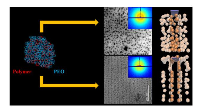
A figure illustrating that polymer crystallization speed can be used to control the spatial distribution of nanoparticles. Impurities (here, the nanoparticles) will become engulfed by the crystal if it grows too rapidly. However, when the rate slows, the crystal will expel the defects. Credit: Sanat Kumar/Columbia Engineering
