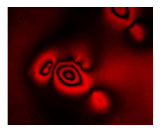
Scientists at the University of St Andrews have developed a new microscopy method that analyses interference patterns to create images of the forces living cells apply as they grow, divide and migrate: shown is the force pattern generated by a human embryonic kidney cell in contact with a probe that is read out by red light. Credit: University of St Andrews
