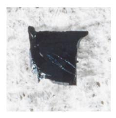
Materials scientists at Argonne National Laboratory synthesized these single crystals of a metallic trilayer nickelate compound via a high-pressure crystal growth process. A team led by John Mitchell, an Argonne Distinguished Fellow and associate director of the laboratory's Materials Science Division, describe the compound's potential as a high-temperature superconductor in the June 12 issue of *Nature Physics*. Credit: Argonne National Laboratory
