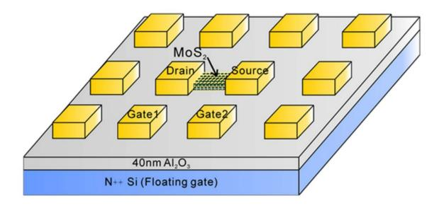
Structure of the neuron transistor, which contains a 2D flake of MoS2. Credit: S. G. Hu et al. ©2017 IOP Publishing
