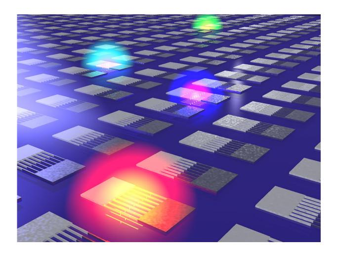
Artist's representation of a conceptual design for the color detector, which uses thermoelectric structures with arrays of nanoscale wires that absorb different wavelengths of light based on their width. Credit: Harry Atwater and Kelly Mauser/Caltech
