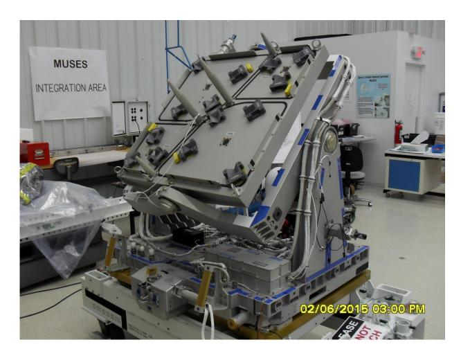
The MUSES platform accommodates up to four instruments simultaneously. Each instrument can be installed and removed robotically by the ISS robotic arm operators on the ground. Credit: Teledyne Brown Engineering
