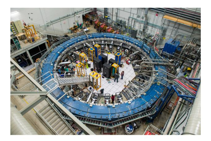
The Muon g-2 electromagnet at Fermilab, ready to receive a beam of muon particles. The ring generates a remarkably uniform magnetic field with which scientists will study properties of the muon in a hunt for undiscovered particles and forces Credit: Reidar Hahn/Fermilab
