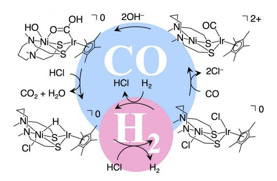
Reaction mechanism with a catalyst for fuel cells that use hydrogen and carbon monoxide as fuels. Credit: Kyushu University
