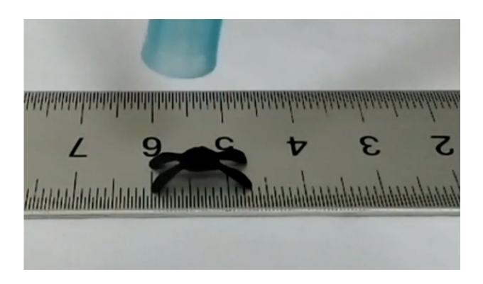
Using an off-the-shelf camera flash, researchers turned an ordinary sheet of graphene oxide into a material that bends when exposed to moisture. They then used this material to make a spider-like crawler and claw robot that move in response to changing humidity without the need for any external power.
