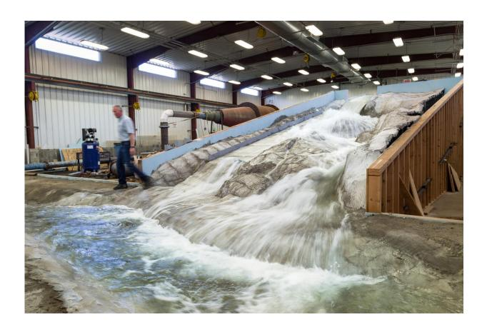
Engineers at the Utah Water Research Lab constructed a 1:50 scale model of the Oroville Dam spillway. Credit: Matt Jensen/Utah State University
