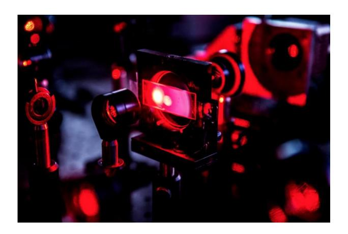
A patterned spot of laser light appears on the slide filled with yogurt. Moussa N'Gom and his team measured the brightness of the light getting through for hundreds of patterns, which their algorithm built into a mathematical representation of the yogurt's scattering pattern. Credit: Joseph Xu, Michigan Engineering
