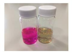
Vials containing the Rhodamine B test dye used in the study, both before (left) and after (right) photocatalytic degradation by the composite under white light illumination. Credit: Daniel Jones/Swansea University
